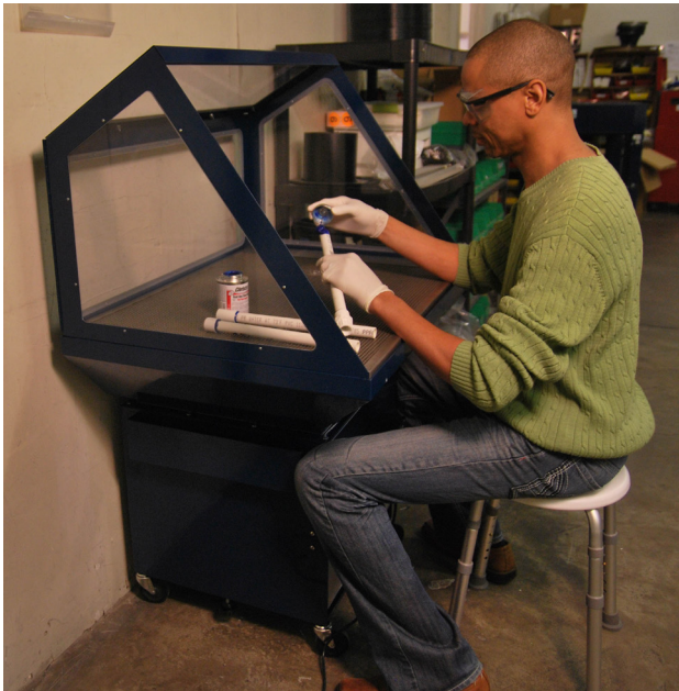
Epoxy gluing shown on sitting version w/ clear doghouse.
