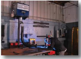
The **Model 400 Stand Mounted Sentry** fume extractor with flex arm is a complete industrial air cleaning system designed for elevated, source-capture fume extraction. This system is equipped with a powerful fan and a variety of inlet collar sizes to match your unique application and also features a variable speed controller and optional remote control.
